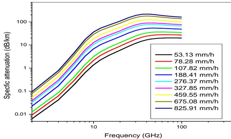
Fig (30): Frequency characteristics of specific attenuation for convective rain type at different rain rates
