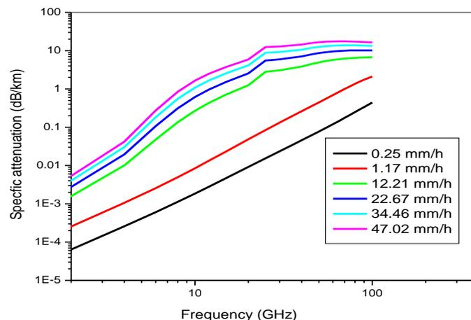
Fig (29): Frequency characteristics of specific attenuation for Stratiform rain type at different rain rates
