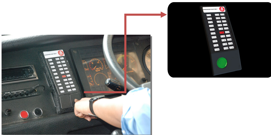
Figure 1.2 : Main sign indicator warning system box.
